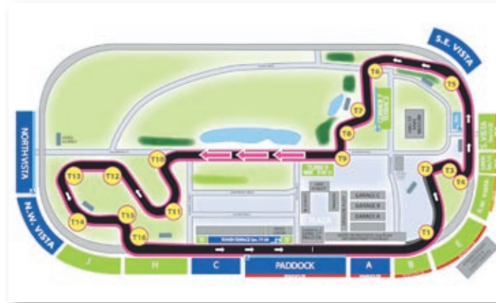
An entirely new 16-turn, 2.6 mile MotoGP motorcycle road course is being built at Indianapolis to utilize select sections of the oval.
