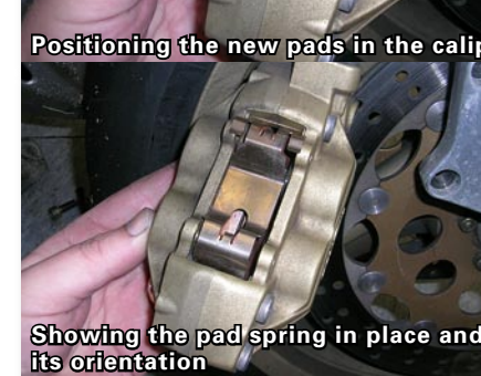
Positioning the new pads in the caliper
