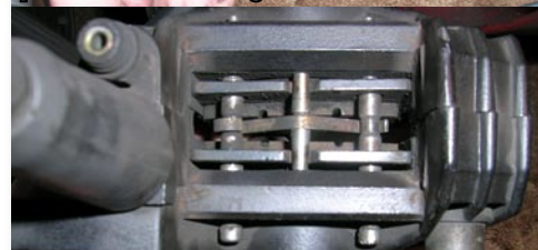
Cover removed and showing the Paso's pad/pin/spring orientation
