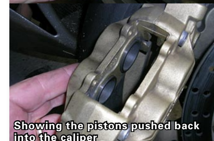
Pushing the pistons into the caliper using the old brake pads and a large screwdriver
