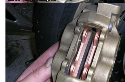
Positioning the new pads in the caliper
