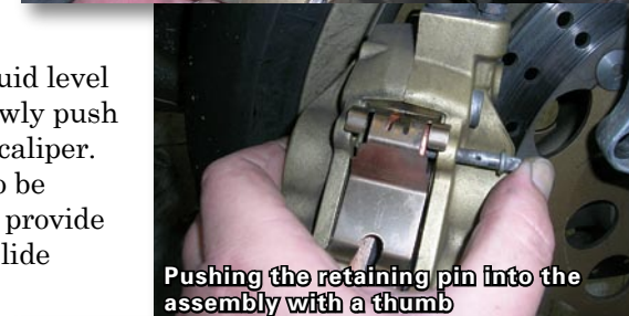
Sliding the first retaining pin back into the assembly
