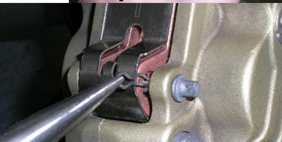
Pushing the retaining pin into the assembly with a thumb
