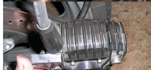
Paso caliper removed and showing the plastic cover hiding the internals
