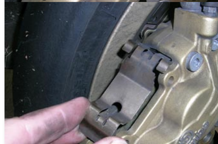
Pulling out the second retaining pin
