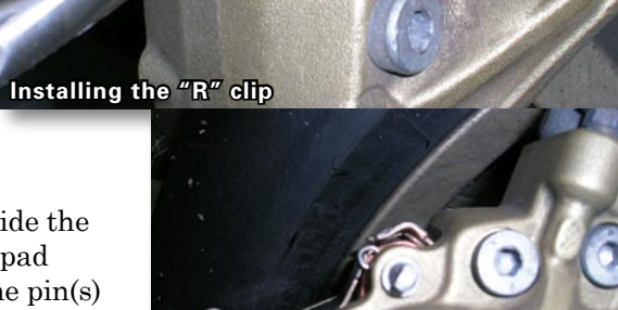
Showing the reinstallation of the "R" clip
