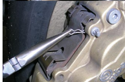
Removing the second "R" clip with needle-nose pliers
