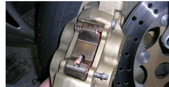
Sliding the first retaining pin back into the assembly
