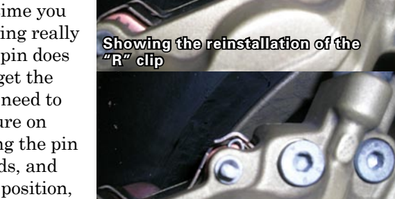
Showing the upper "R" clip position once back in the caliper
