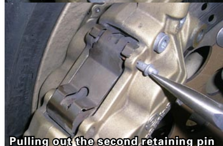
Removing the second "R" clip with needle-nose pliers
