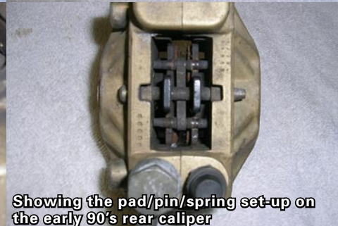
An early 90s single-pin compression fit rear caliper from a '94 900SS
