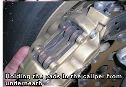
Showing the orientation and removal of the pad spring
