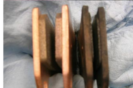
Removing the used pads from the bottom of the caliper
