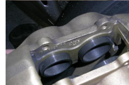
Cleaning inside the caliper and exposed pistons with an old toothbrush
