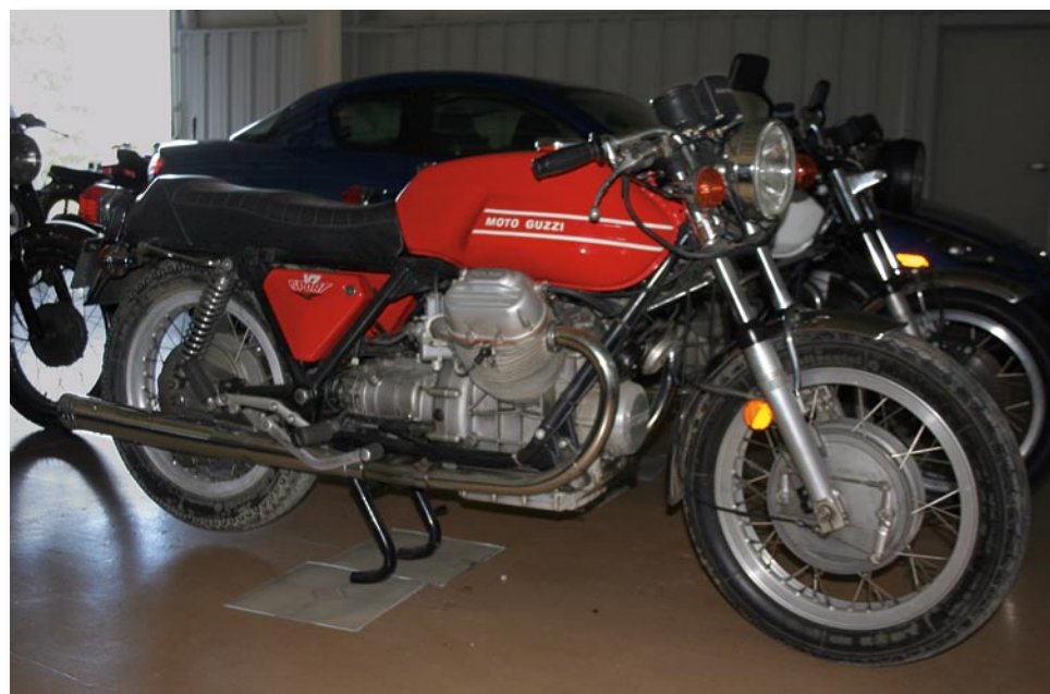
A four-leading-shoe drum brake Moto Guzzi V-7 Sport
