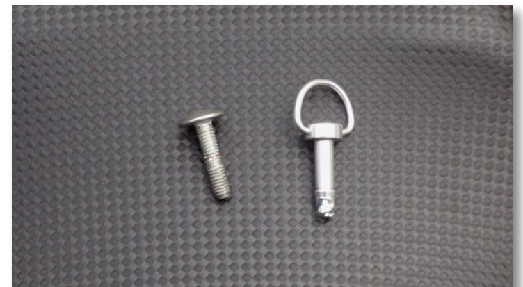
Stock bolt side by side with new Dzus fastener
