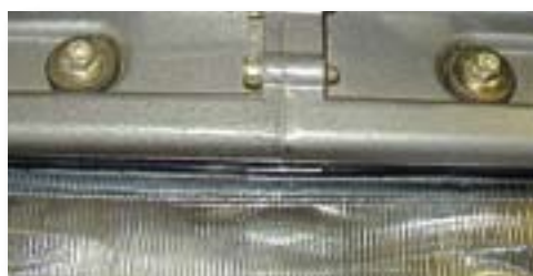
Photo 3. Upper Headlamp Bolts
