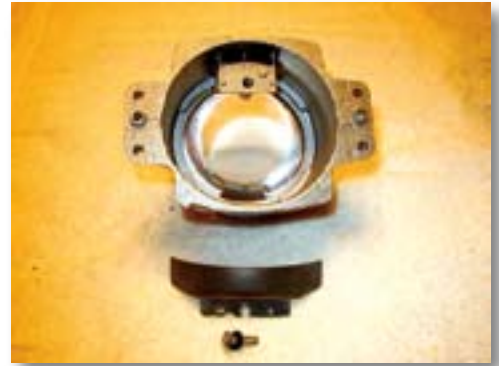
Photo 13. Removed Low-Beam Cut-Off Plate
