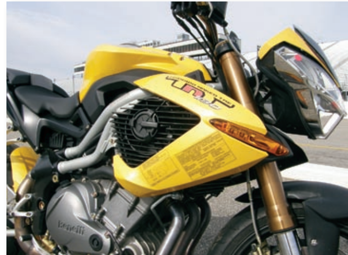
The engine on the Tre is a beautifully crafted of a mill that is made by Benelli, not an import manufacturer. Dual radiators are side-mounted with thermostatically controlled fans that pull air through - and out. Oil-cooler is center mounted between the transformer like side panels. J. Rossi Photo courtesy VivaDUCATI.com
