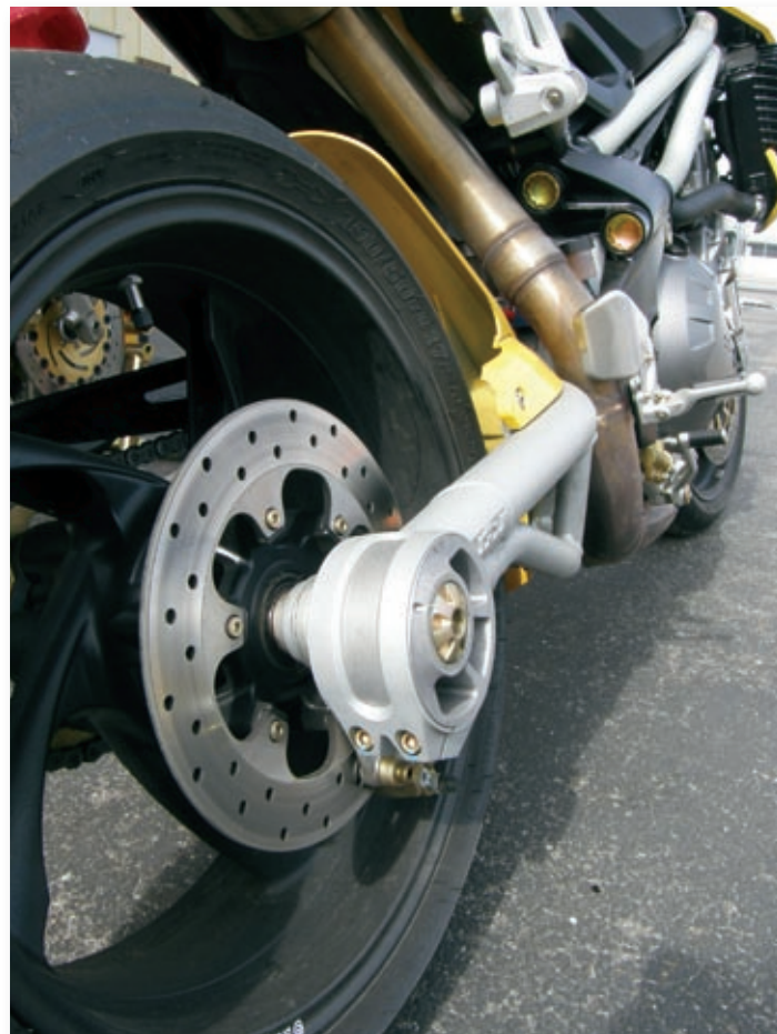
This magnificently over-sized concentric axle/ chain adjustment is so brilliantly bizarre yet functionally accurate compared to the tiny watch-like adjusters that most of us have tolerated for years. You have to wonder if adjustments change the ride height. From this vantage point, you can see how the dual steel frame tubes are received into the cast aluminum engine mount with recessed, gold anodized, triple square (XZN) socket bolts used in high torque applications. J. Rossi Photo courtesy VivaDUCATI.com
