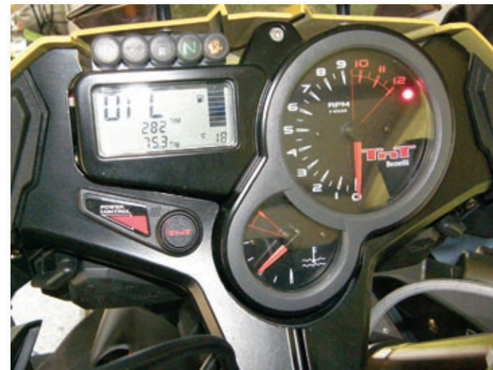
Instrumentation is a welcome combination of a sweeping hand-tachometer and temp gauge both - easy to read, with the all too common etch-a-sketch, grey-on-grey speedo, fuel capacity, trip-meter. The “Power Control” button is an on-the fly, econo, self imposed traction control. Go from exotic Italian performance to an the feel of an EX500 with a sock in the intake with a touch of a button. A little gimmicky at first but completely useful in heavy, consistently paced traffic and wet conditions. J. Rossi Photo courtesy VivaDUCATI.com
