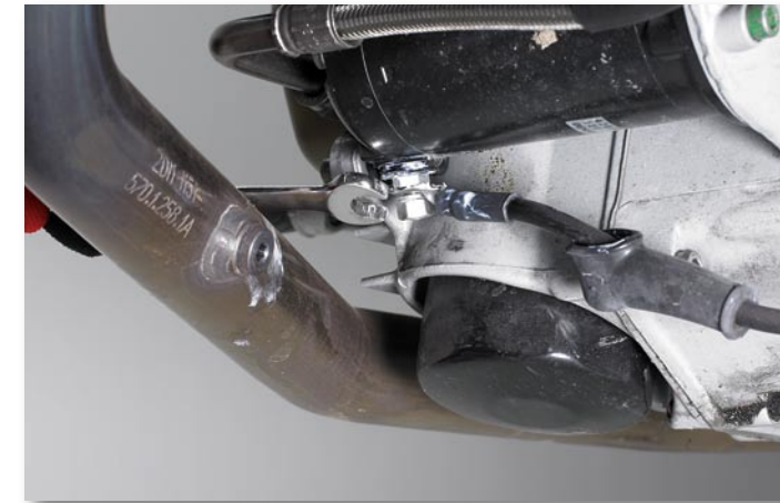
This is the old starter cable which will not be your ground. Be sure to tag the end of the new starter cable so when you go to hook up the cables at the battery you will not get confused and reverse them.
