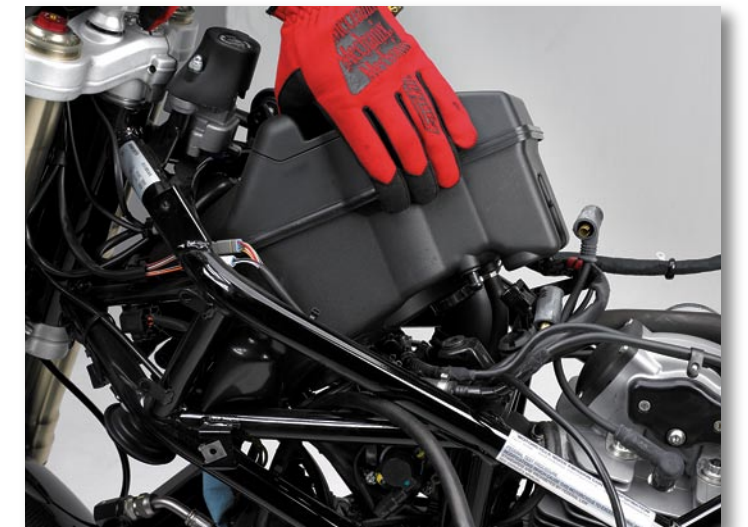
This is the air box and where most of the new tank volume comes from
