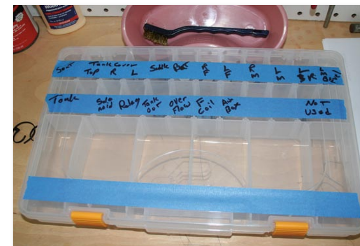
I label each bolt and part removed so there is no doubt where it goes.
