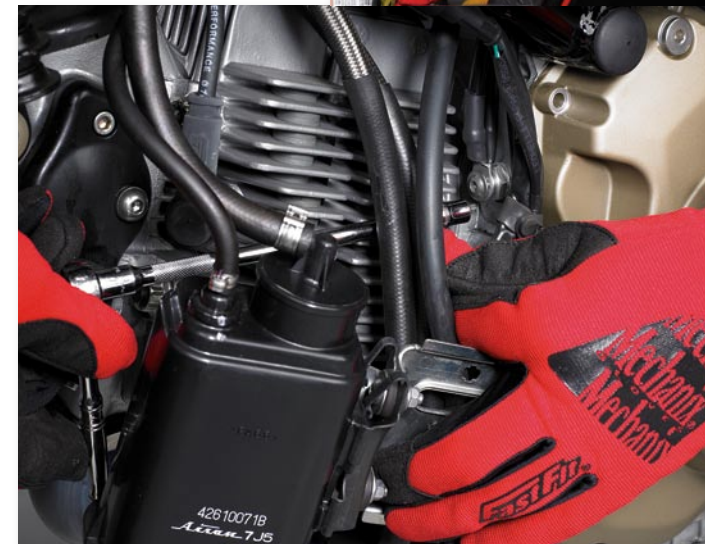
This is the old ground cable where the old starter cable will go. Be sure to get your ground tight many electrical problems can start here.
