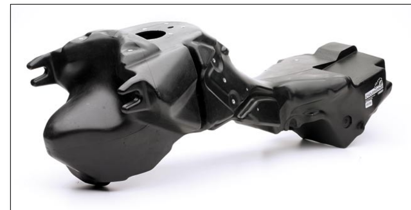
Note the large area in front of the Cycleworks’ tank where the air box used to be. In the rear you can see the battery area on the left rear section is filled in and there is a smaller recess on the top where the battery now resides.
