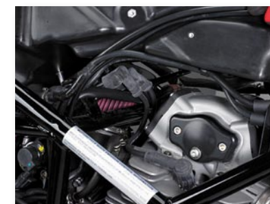
The red individual air filters in place.
