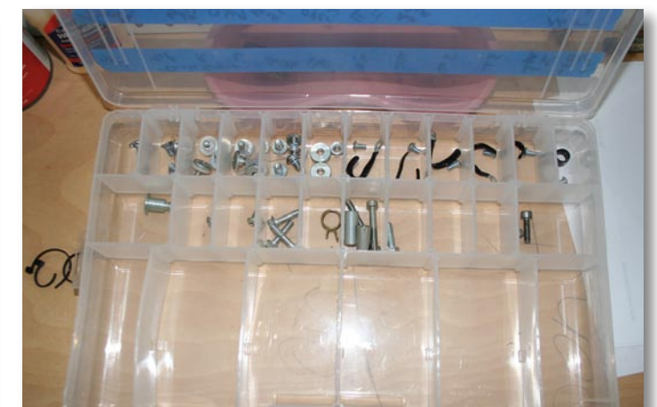
Each part has its own bin including the ones that are not to be reinstalled. This is how I knew where the left over bolt went. :-)
