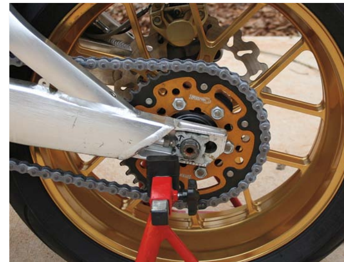
Composite sprocket, not as light as full aluminum but it lasts a lot longer.
