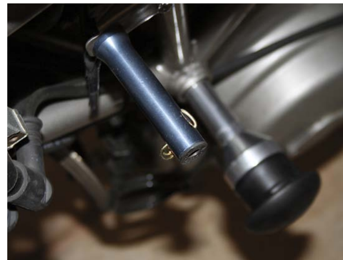
Wellnut conversion to a Dzus fastener; the frame slider has since been removed by order of Fast Frank.
