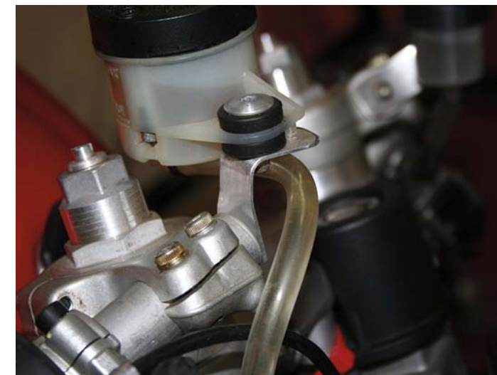
Fabricated reservoir mount installed on inside end of bars. Clear brake hoses to prevent bubbles.
