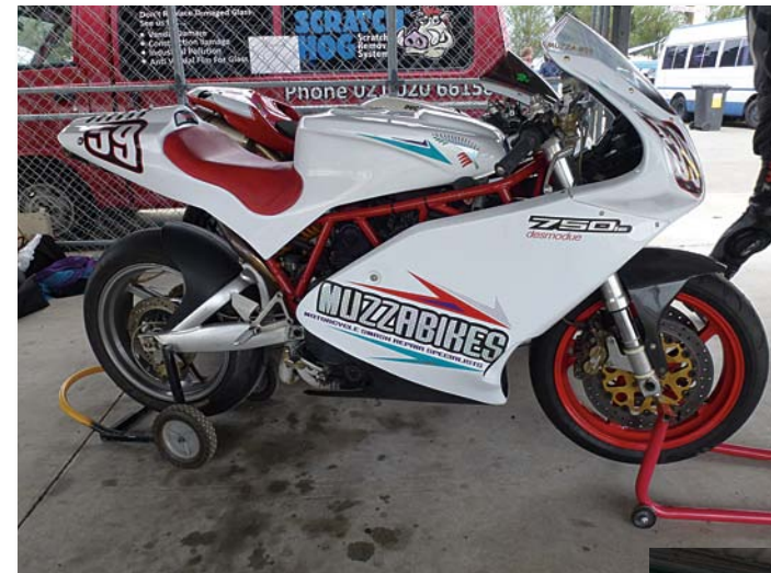
Murray's 750 super stock showing the fiberglass tank-seat combinations he builds
