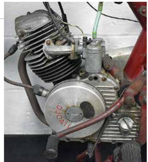
While many small displacement motorcycles of the day were 2-strokes, the Ducati 60 was a 2.25-horsepower, 4-stroke powerhouse.
